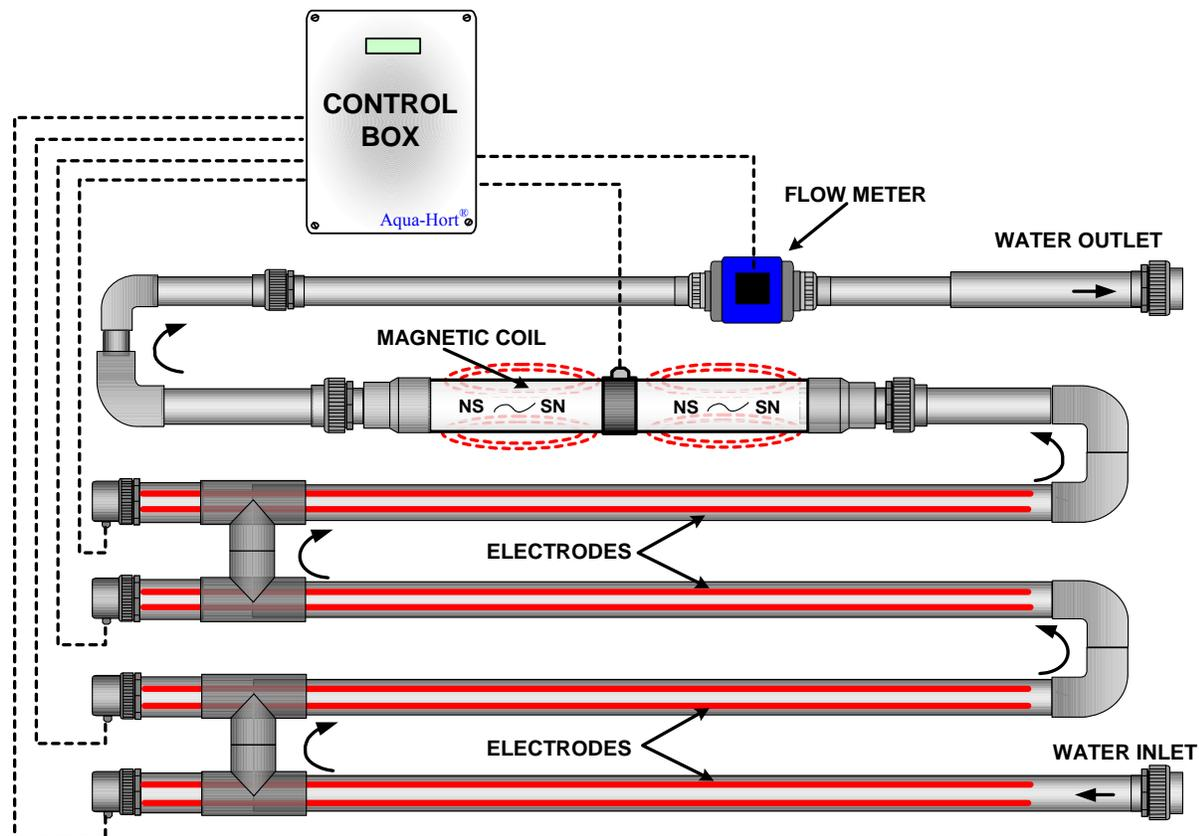
**Figure 9.1.** This AquaHort copper system is equipped with copper electrodes inside pipes. An electrical current passes through the system to turn solid copper metal electrodes into soluble copper ions. A magnetic coil increases activity of the copper ions. The control box corrects ionization rate based on water flow and water electrical conductivity to maintain a constant copper concentration.
