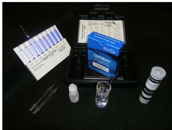
**Figure 8.4. Peroxyacetic acid concentration can be measured with a colorimetric test kit or test strips.**
