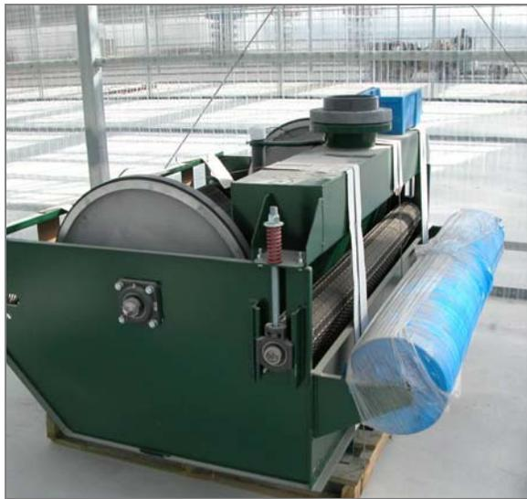
**Figure 3.4.** A paper filter ready for installation into a flood floor greenhouse.
