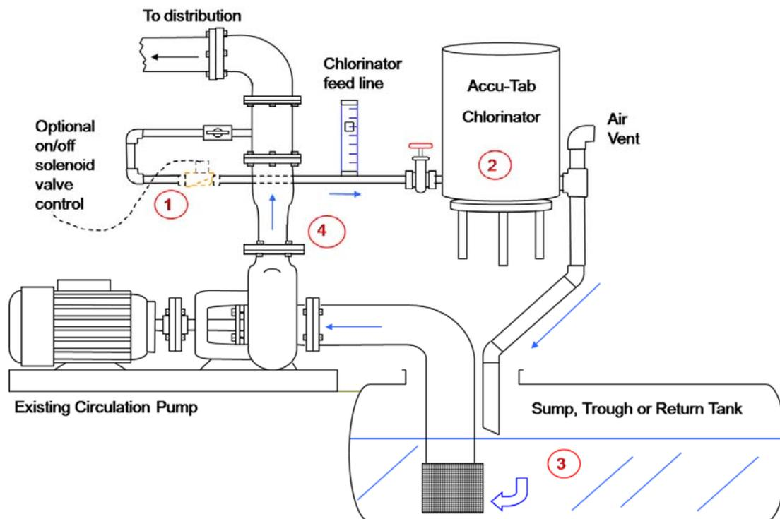
**Figure 5.4. System diagram for calcium hypochlorite.**
