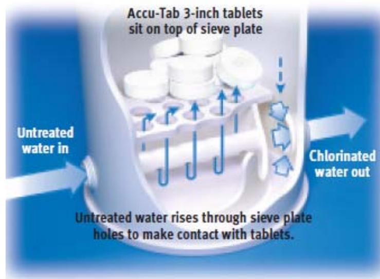
Figure 5.3. Diagram of a calcium hypochlorite chlorinator.
