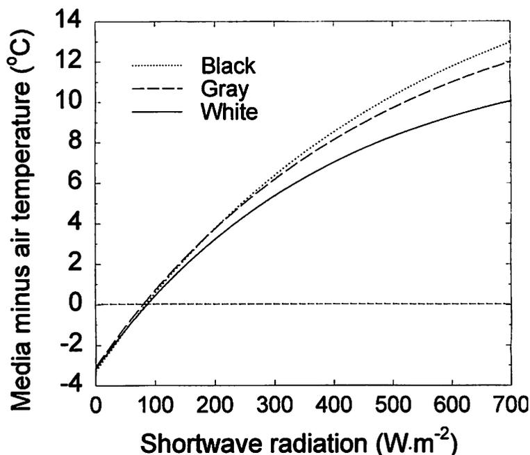
**Fig. 2.** The effect of plug-flat color on medium-surface temperature shown as a function of the incident solar radiation (280 to 3000 nm). Air temperature was maintained at 25 °C and the water vapor pressure deficit averaged 1.4 kPa.
